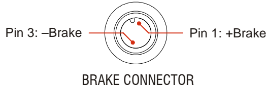
Figure R1.11 M12 Brake Connector Pinout
