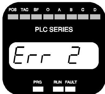
Fig 2.19 E 2 PROM Fault
