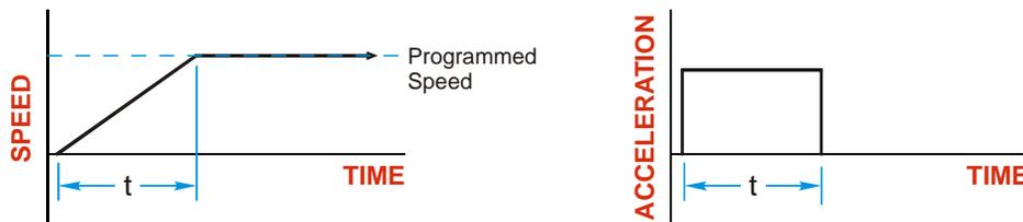
Figure 2.1 Linear Acceleration
