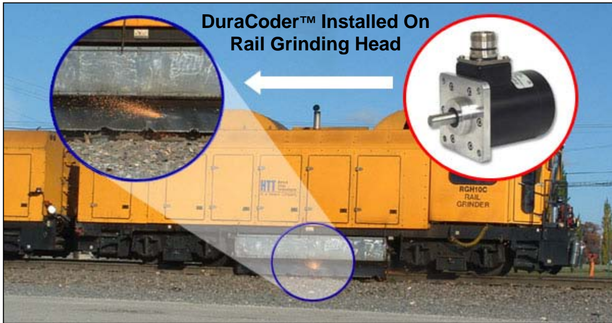
AMCI DC25 Analog DuraCoder™ Mounting Location On Harsco RGH10C Rail Grinder
