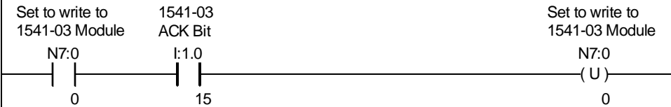
Figure 3.3 Sample Ladder Logic Program
