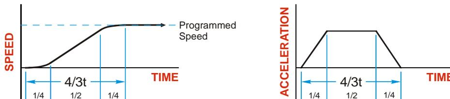
Figure 2.4 Trapezoidal S-Curve Acceleration
